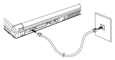
Connecting the internal modem
